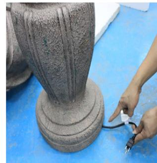
Align the pump cord with the groove at the base of the pedestal.
