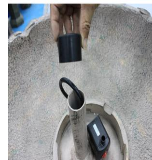
Install the cord pipe cover over the cord pipe. Attach the tubing to the pump.
