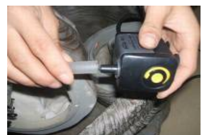
Connect tubing of top part to the pump
