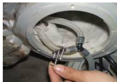
Use restrictor to help control water flow to the top
