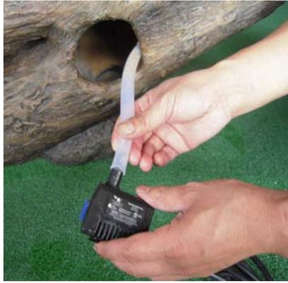
Locate the tubing from inside the fountain and connect it to the pump. Adjust the flow control as needed.
