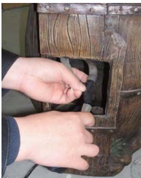
Install the "Y" joint. Then connect tubing of pump to it.
