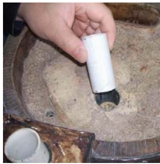
Insert another PVC into place
