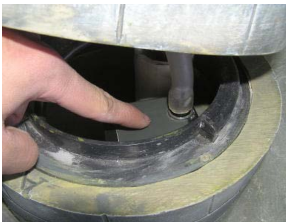
Add top, be sure pump sits at bottom and hose does not bend. Secure using twist and lock. Cord out back of the unit.
