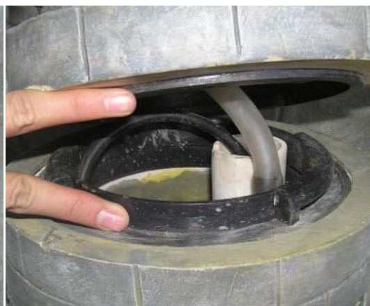
Add top, be sure pump sits at bottom and hose does not bend. Secure using twist and lock. Cord out back of the unit.
