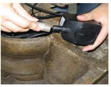
Connect the tubing from the top to the pump as shown above.
