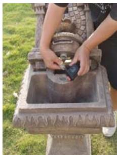
Connect the tubing from the top to the pump, and place the pump inside the water reservoir.
