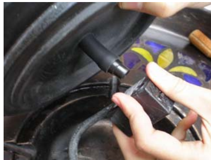
Connect the output to the pump tightly.
