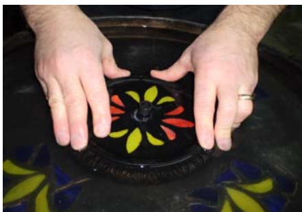
You may need to rotate the plate in either direction to help the pump and nozzle sit better in place.
