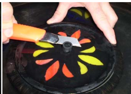
If you wish to alter the bubbling height, the tubing can be trimmed as needed as shown above.
