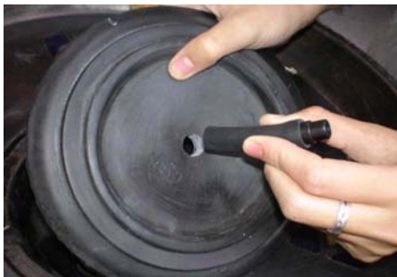
Feed the tubing through the opening in the plate.
