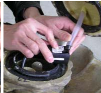
place outlet into tubing outlet into pump
