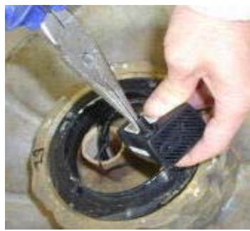
pull pump outlet out with pliers
