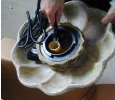
cord through standpipe
