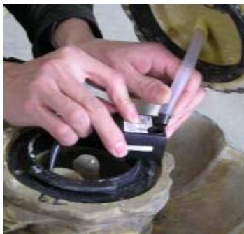
place outlet into tubing outlet into pump
