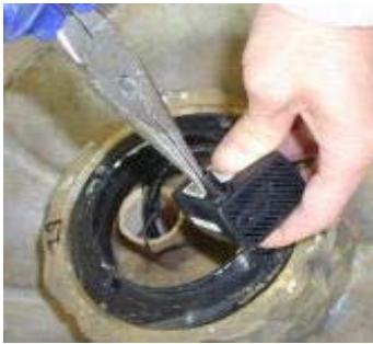
pull pump outlet out with pliers
