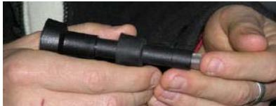
Insert the small piece of tubing (supplied) in the spray nozzle tube as shown. Be sure to get in straight. This will reduce the spray height and reduce water loss.
