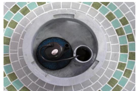
For solar pump, attach filter on bottom. Chosen pump must be centered in cavity.
