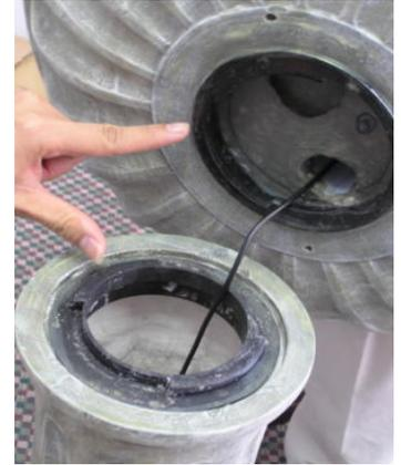
The power cord is inserted through the pipe in the bowl as shown. Cord must then be fed through pedestal and out grooved notch at bottom. Secure bowl and base together using the twist and lock assembly system, noting the position of the grooves.
