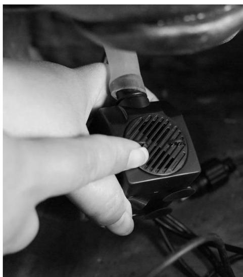
The pump is set to full strength, adjust as needed. Place the pump inside the reservoir. Any excess cord can be retrieved out the back of the fountain.
