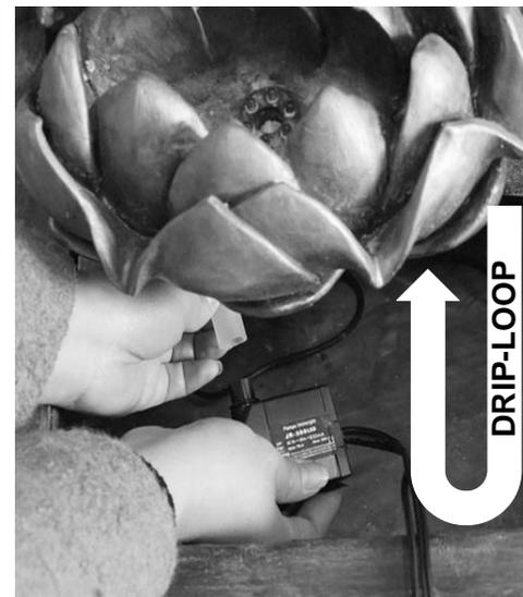
To prevent the chance of water loss, ensure the cable from the light has a drip loop before it exits out the rear.
