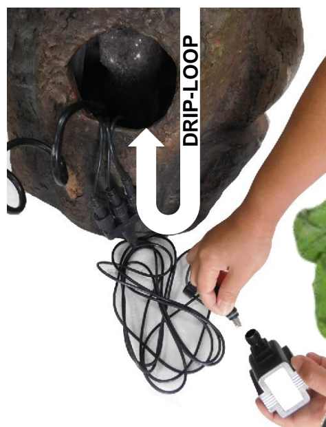
Connect the cable from the connector to the transformer. IMPORTANT: to prevent water loss, create a drip-loop with the light cables by dipping them into the reservoir before they exit out the back of the fountain.
