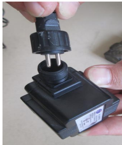
Securely attach the light cord to the transformer.
