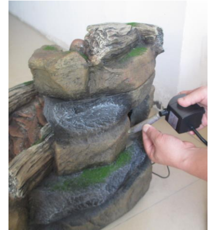
Locate the tubing from inside the fountain and attach it to the pump.
