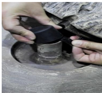
IMPORTANT: To prevent the chance of water loss during operation, install the cord pipe cover over the cord pipe as shown above.
