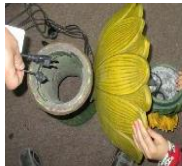
Pass the cord from the connector and the pump cord down the pedestal and out the base. Align each of the cords with the groove in the base of the pedestal. Securely attach the cord from the light to the transformer.
