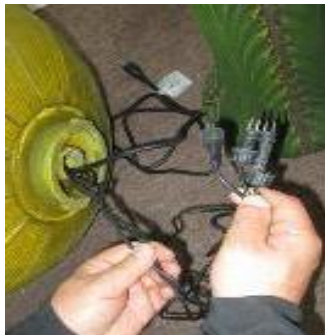
Carefully position or hold the top and bowl for safety. Once all light cords have passed through the bowl, securely connect them to the 3 to 1 connector.
