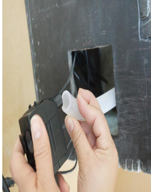
Locate and attach the tubing to the pump. Water flow can be adjusted using the control on the front of the pump.
