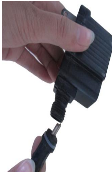
Attach the cord from the connector to the transformer.
