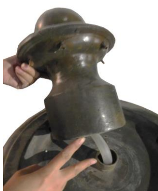
Attach the tubing to the top. Pass the tubing from the top through the small bowl and into the riser.
