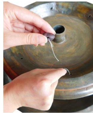
Optional: the splash line can be passed through the spill pipes to reduce splash and sound.
