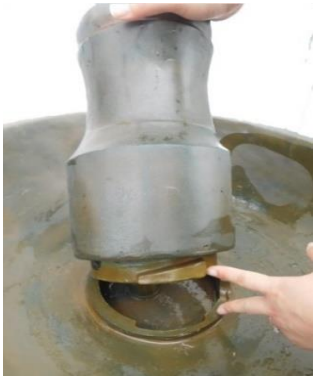
Align and lower the riser over the pump and on to the large bowl. Turn clockwise to lock in place.
