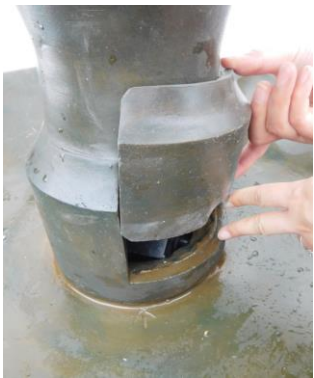
Align and install the pump access door.
