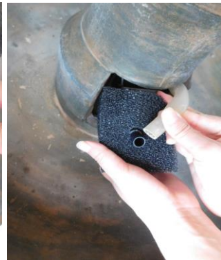
Retrieve and attach the tubing to the pump.
