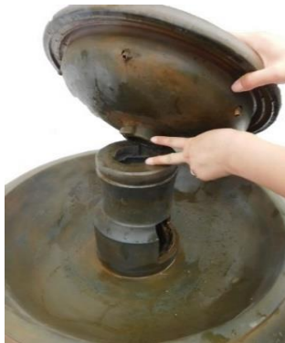
Align and lower the small bowl on to the riser. Turn clockwise to lock in place.
