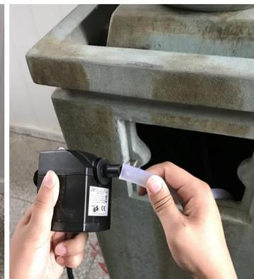
Locate the tubing through the pump access door. Attach the tubing to the pump.
