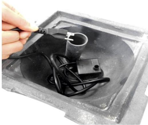
Place the pump inside the reservoir then pass the power cord down the cord pipe.
