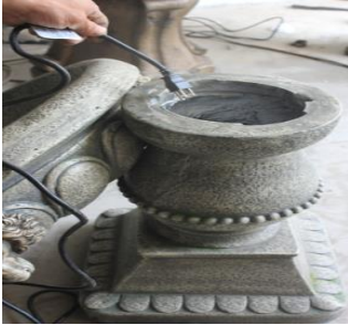
Carefully rest the bowl on its side. Feed the pump cord down the pedestal and out the base.
