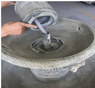
Feed the tubing up and through the riser.
