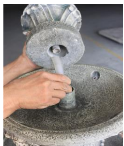
Connect the tubing to the top.
