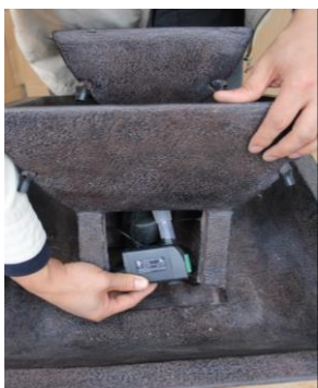
Attach the tubing to the pump. Position the pump inside the reservoir as shown.
