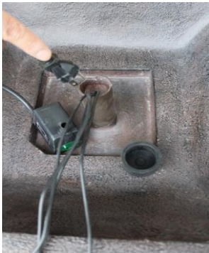
Pass the cord from the pump down the cord pipe in the bowl.
