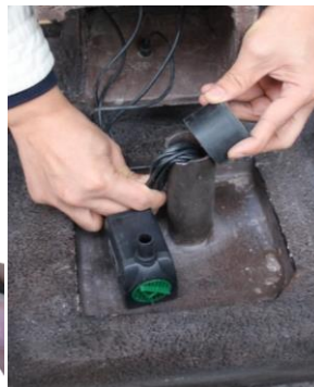
Install the cord pipe cover over the cord pipe.
