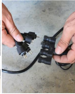
Attach the light cords to the connector.
