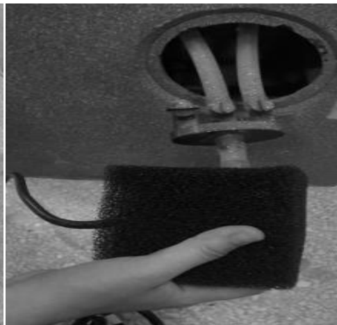
Locate the tubing from inside the fountain and attach it to the output of the pump. To fine-tune water flow, the controls can be adjusted on the diverter as needed.
