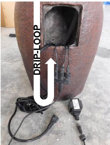
IMPORTANT: to prevent water loss during operation, create a drip-loop with the 3 light cords by dipping them into the reservoir before they exit out the back of the fountain.
