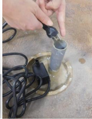
Pass the power cord from the pump down the cord pipe in the large bowl then down the pedestal.
