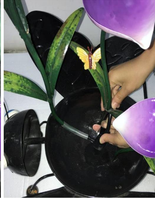
Place the pump inside the fountain. Water flow can be adjusted using the dial on the front of the pump.
