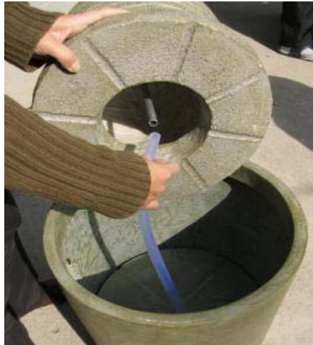
Attach tube to metal pipe
