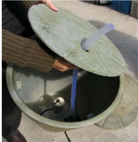
Sit pump at bottom, slide tube through baffle plate as shown.
