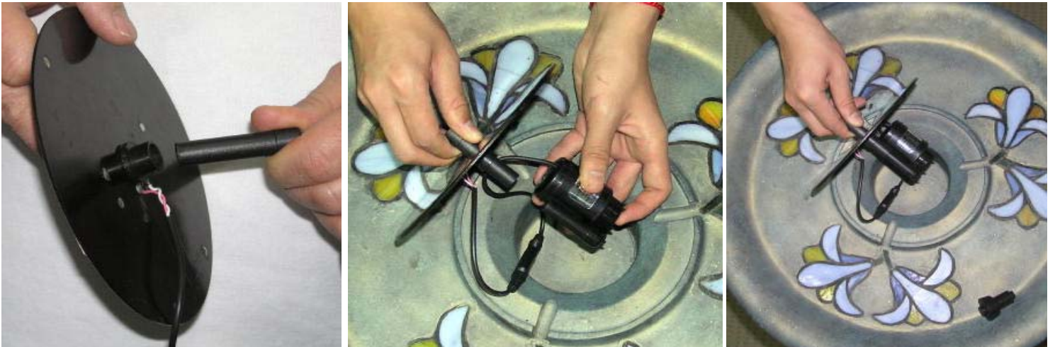
Insert pipe into panel from bottom. Attach tube to pump.
