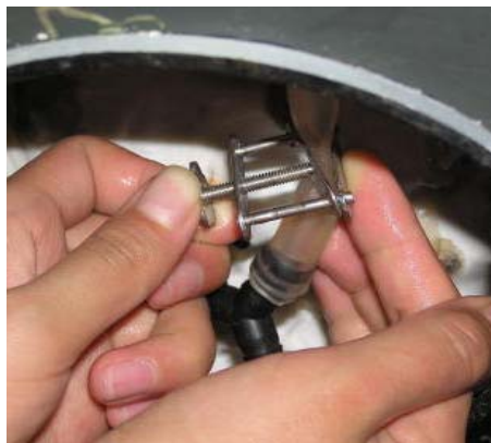
Place pump in bucket and run cor through notch. Restrictor is included for fine tuning flow. Place pump outlet into tubing.
