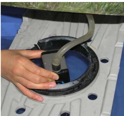
Insert tubing into pump.
