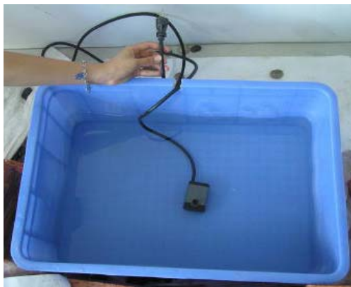
Place pump in bucket and run cor through notch. Restrictor is included for fine tuning flow. Place pump outlet into tubing.
