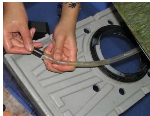
Place pump in bucket and run cor through notch. Restrictor is included for fine tuning flow. Place pump outlet into tubing.
