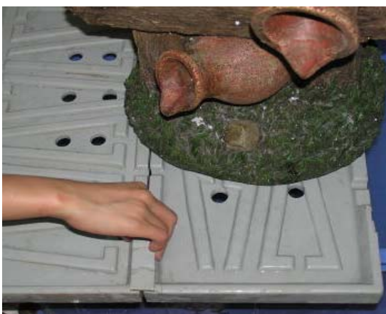
Side plates set on bucket using grooves.
