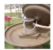
Carefully rest the second bowl on its edge and pass the tubing up through it as
