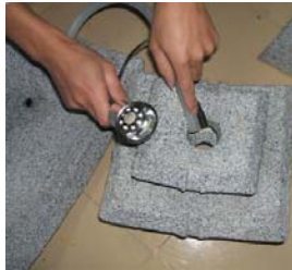
Pass the light cord and tubing through the opening of the top piece and press the light in place. Pass the tubing and light cord through the middle of the largest bowl as shown.
