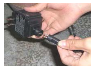
Attach the cord to the transformer. Ensure it is tight. Place the transformer in a safe area, preferably under cover. While this unit is rated for outdoor use, it should not be fully submerged in the water.
