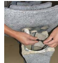
Connect the tubing to the pump and attach the cord from the light to the pump. Be sure it is secure.
