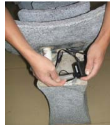
Connect the tubing to the pump and attach the cord from the light to the pump. Be sure it is secure.
