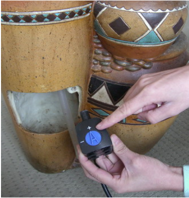
The pump is set to full strength. If splash is a concern, adjust the flow as needed.
