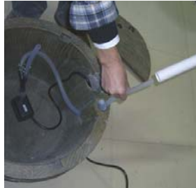
Feed the longest piece of tubing up through the access hole to the top as shown.
