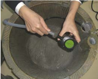
Connect the end with the shortest piece of tubing to the pump.
