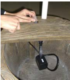
Feed the remaining tube up through the hole in the plate as shown.
