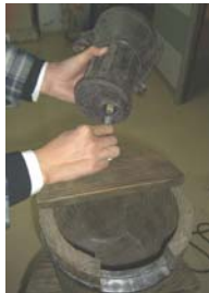
Connect the tubing to the top feature. Set the top into place by sliding it over the white pipe.
