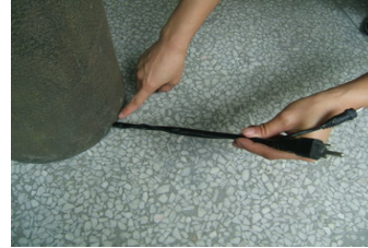
Feed the pump and light cord through the cordpipe in the base. Align the cord with the groove at the base.
