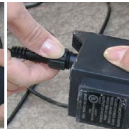
Attach light cord to transformer. Be sure it is tight. Place transformer in a secure area, preferably under cover. While this unit is rated for outdoor use, it should not be fully submersed in the water.
