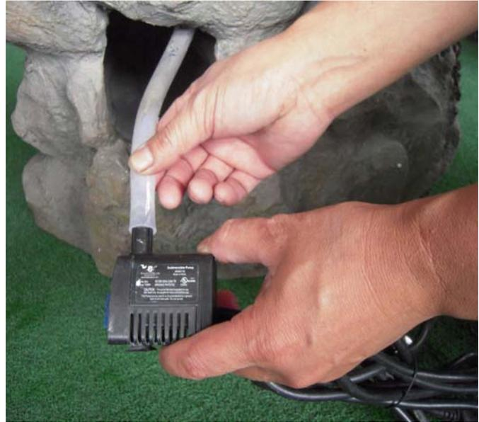
Locate the tubing from inside the fountain and connect it to the pump. The pump is preset to full strength, if splash is a concern adjust the flow control as needed.
