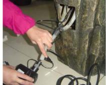
Connect the tubing to the pump and adjust the pump to its highest setting.
