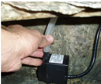
Connect tubing to the pump.
