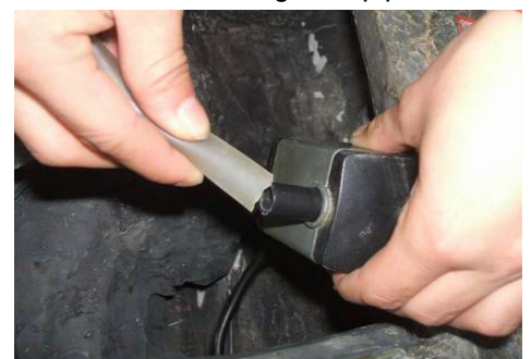
Feed the tubing through the pipe.
