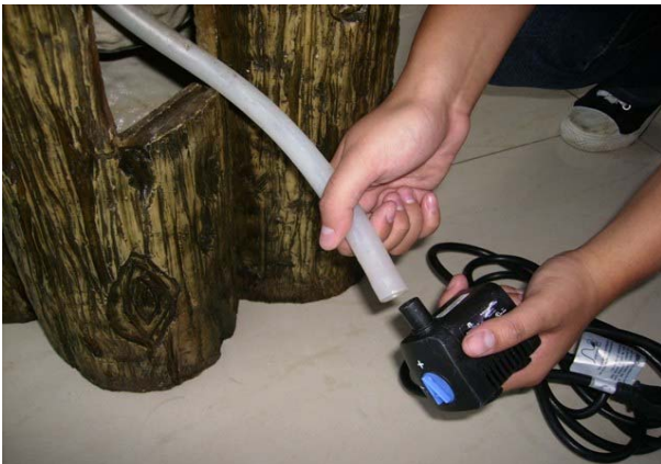
Connect the pump to the tubing and adjust the pump to your desired setting.
