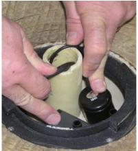
Pump cord through pedestal into groove at bottom. Twist and loct bowl to pedestal, note the proper tree branch line up.
