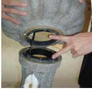
Attach the bowl to the base using the twist and lock assembly system. Note the position of the grooves.
