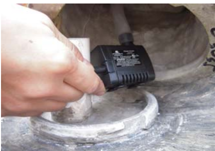
Place the pump flat inside the reservoir. Lower the top over the pump and twist and lock it to the bowl. Ensure the tubing is not kinked or interfering with the assembly.
