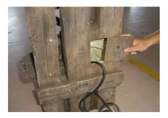
After placing the pump inside the reservoir, slide the pump access door into place.
