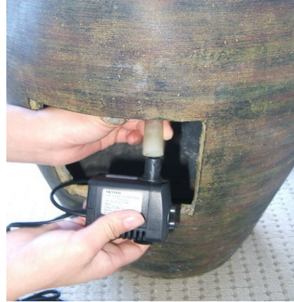
Connect the tubing to the pump and place pump inside the fountain
