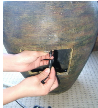
Connect the tubing to the pump and place pump inside the fountain
