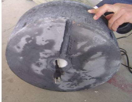
Feed the pump cord down through the cord pipe and align with groove at the base.
