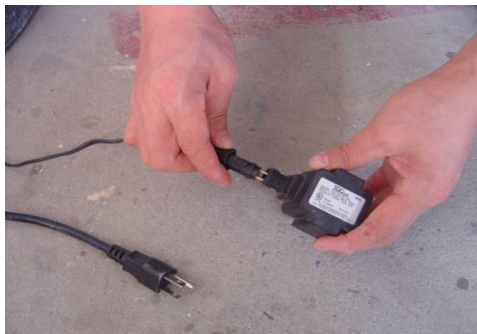
Attach light cord to transformer. Be sure it is tight. Place transformer in a secure area, preferably under cover. While this unit is rated for outdoor use, it should not be fully submersed in the water.
