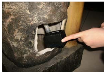
Place the pump inside the reservoir being certain it is fully submersed, sitting flat and the tubing is not kinked.
