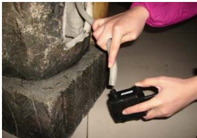
Connect the tubing to the pump. Adjust the pump to full strength. If splash is a concern, adjust the flow control as needed.
