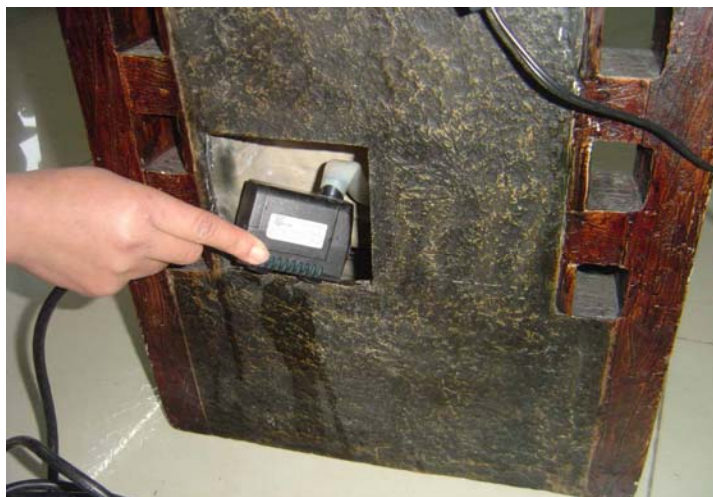
Place the pump inside the reservoir, being certain it is fully submerged and sitting flat on the base.
