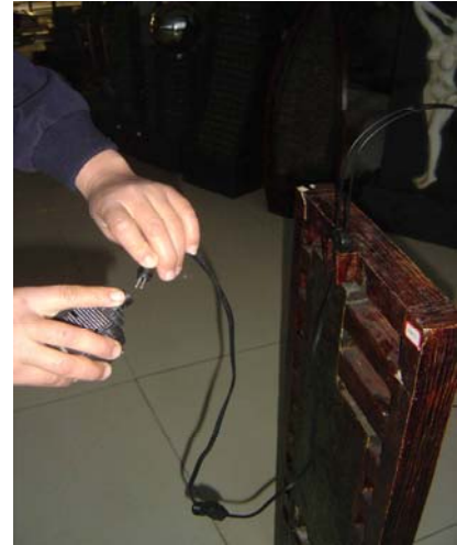
Connect the cord from the light to the transformer.
