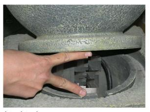
Attach tubing to pump, twist and lock top into place.
