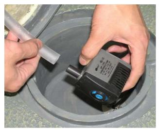
Pump is pre installed. Note flow control to adjust. We recommend full strength setting for maximum effect, but you may want to adjust downward in areas where splashing is a concern.
