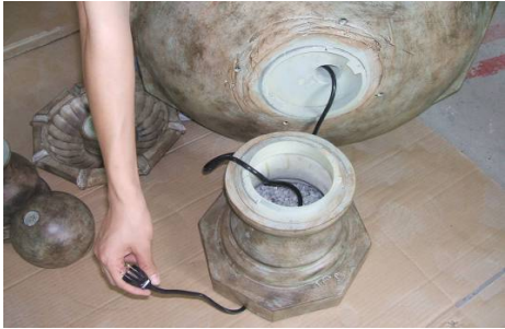
Run cord through leg as illustrated. There is a groove in the base of the leg for the cord.
