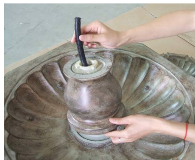
"Twist and lock" riser in place.
